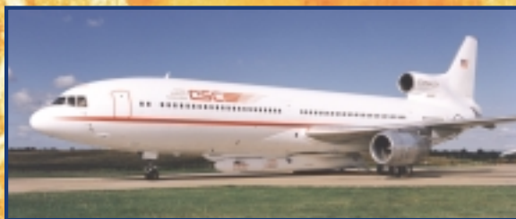
The Marshall modified L10-11 TriStar carrying the Pegasus Satellite Launch Rocket.
